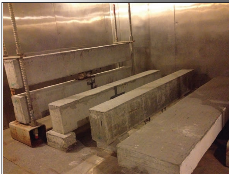
Figure 1. Beams inside Environmental Chamber
